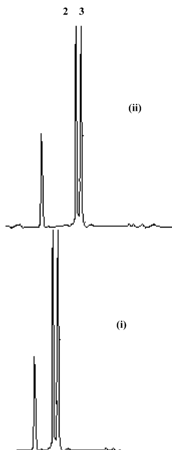
Fig. 6. Comparison of chromatograms obtained after injecting the extract obtained from deproteinated plasma fortified with 0.5 \text{ mg L}^{-1} Tyrosine and 0.5 \text{ mg L}^{-1} phenylalanine (i) following batch extraction and (ii) on-line approach into the HPLC system. Order of the chromatographic peaks 2: Tyrosine, 3: Phenylalanine. Chromatographic conditions: 60% acetonitril/40% 0.005 M aqueous \text{H}_2\text{SO}_4 ( q=0.4 \text{ mL min}^{-1} ). Detection at 280 nm.
